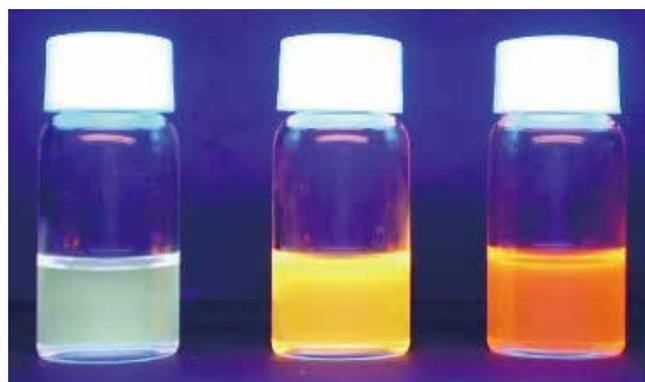
Luminescence from impuritydoped semiconductor nanoparticles.
