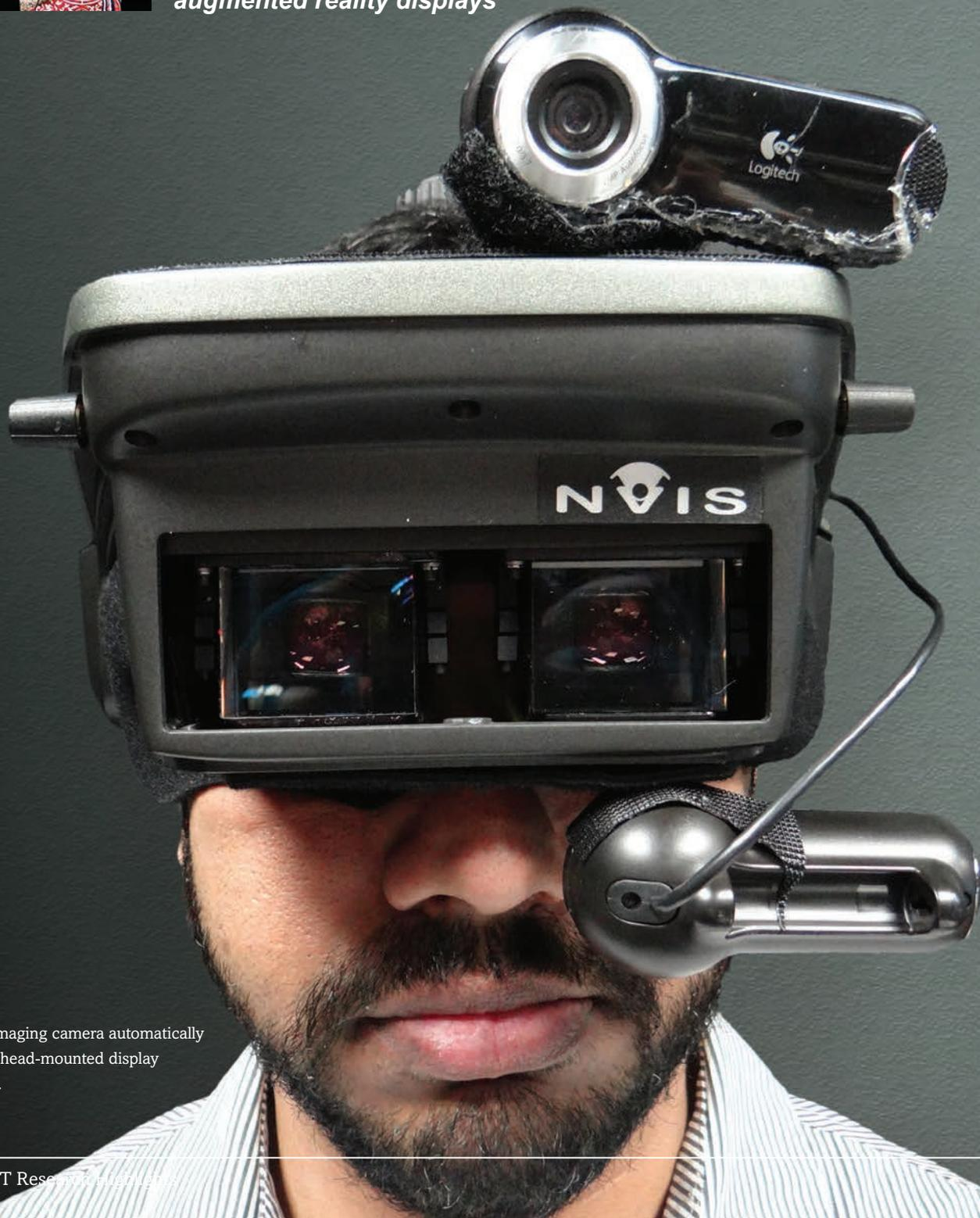
The eye-imaging camera automatically keeps the head-mounted display calibrated.
