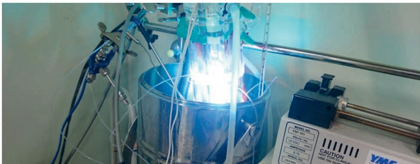
The photoreactor used to produce cyclobutanes.
